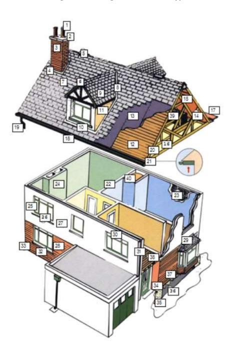
Chimney pots Coping stone 3 Chimney head 4 Flashing Ridge ventilation 5 Ridge board Slates/tiles 8 Valley guttering 9 Dormer projection 10 Dormer flashing 11 Dormer cheeks 12 Sarking 13 Roof felt 14 Trusses 15 Collar 16 Insulation 17 Parapet gutter 18 Eaves guttering 19 Rainwater downpipe 20 Verge boards / skews 21 Soffit boards 22 Partition wall 23 Lath / plaster 24 Chimney breast 25 Window pointing 26 Window sills 27 Rendering
