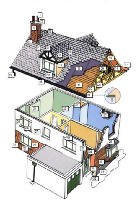
Coping stone 3 Chimney head 4 Flashing Ridge ventilation 5 Ridge board Slates/tiles 8 Valley guttering 9 Dormer projection 10 Dormer flashing 11 Dormer cheeks 12 Sarking 13 Roof felt 14 Trusses 15 Collar 16 Insulation 17 Parapet gutter 18 Eaves guttering 19 Rainwater downpipe 20 Verge boards / skews 21 Soffit boards 22 Partition wall 23 Lath / plaster 24 Chimney breast 25 Window pointing 26 Window sills 27 Rendering 28 Brickwork / pointing 29 window Bay projection 30 Lintels
