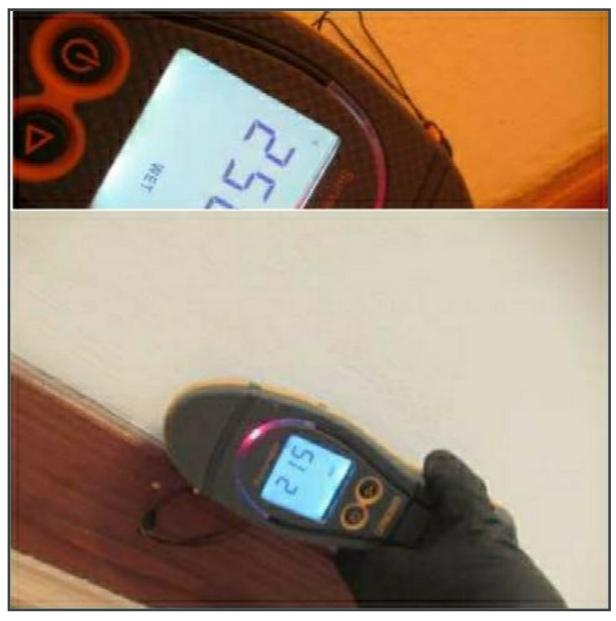
Our inspection of the internal wall surfaces of the property was carried out by a visual inspection and by the use of an electrical conductivity meter; this indicated slightly elevated moisture readings to be present in the walls of the Entrance Hall, Kitchen & Rear Bedroom as highlighted on our enclosed sketch plan and photos.
